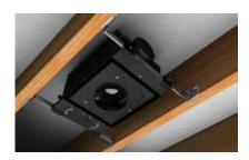
Step 1. Install Aculux new construction housing and gypsum board ceiling per the instruction sheet shipped with the recessed housing. Confirm the ceiling cutout dimensions are either 4-3/8" diameter for round apertures or 4-1/4" x 4-1/4" for square apertures. The aperture must be centered in this cutout to produce a uniform 1/8" gap between drywall and recessed housing.
