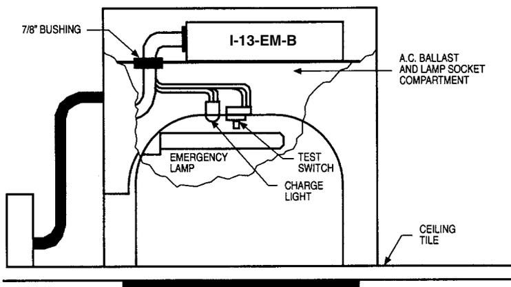
NOTE: Position the Charge Indicator so that it can be seen after installation.
