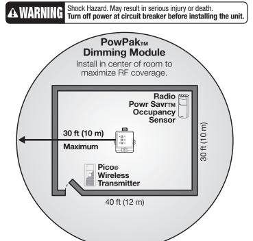
All Wireless Transmitters must be installed within 30 ft (10 m) of the PowPak™ Dimming Module.
