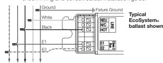
Install PowPakm **Dimming Module**
