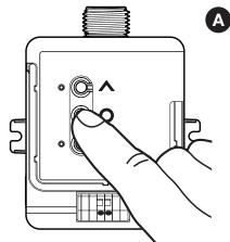
A Hold All On "O" for 6 seconds on PowPak™ **Dimming Module** until ballasts flash. Hold the indicated button on each transmitter for 6 seconds. All ballasts will flash to show Wireless Transmitters have been associated.
