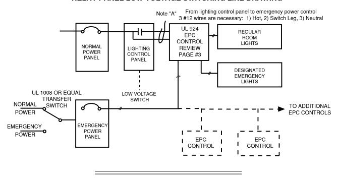
On a 20 Amp circuit, 1 emergency power control (Model EPC) can control up to 16 Amp of emergency lighting load, or 16 emergency power controls can each control 1 amp of emergency lighting load.
