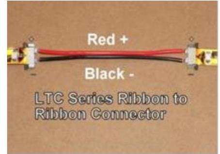
Align polarities and slide ribbon into connector and seat ribbon in fully and push the wedge in fully. (LTC-12",) ribbon to ribbon
