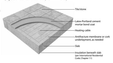
Thick-set mortar bed over slab
