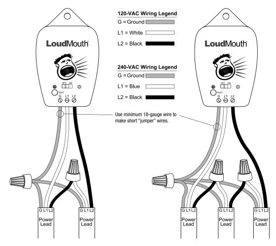
Illustrations showing (left) how to connect the LoudMouth monitor to two cables, and (right) how to connect the LoudMouth to three cables. The LoudMouth can monitor no more than three cables simultaneously. Do NOT leave the power leads connected in "series" like this when making final wiring connections; the cables will not heat sufficiently.
