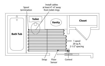
Master Bathroom (normal heat loss, framed floor construction)
