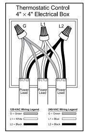
Illustration showing how to connect three cables at the control electrical box.
