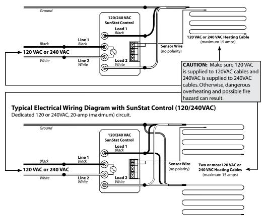
All electrical work must be done by a qualified licensed electrician in accordance with local building and electrical codes, and the National Electrical Code (NEC), especially Article 424, Part IX of the NEC, ANSI/NFPA70 and Section 62 of CEC Part 1.
