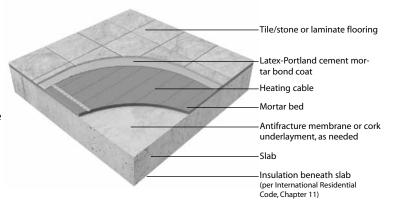
Self-leveling mortar over slab on grade
