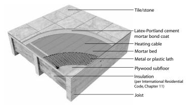
If plastic lath is used instead of the typical metal lath, the cable can be installed before pouring the self-leveling mortar bed.
