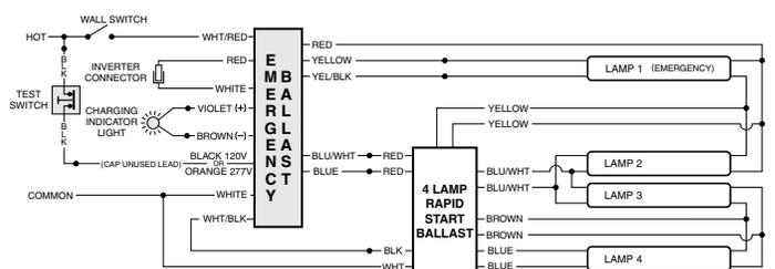
**WIRING DIAGRAMS for Emergency-Only fixtures**
