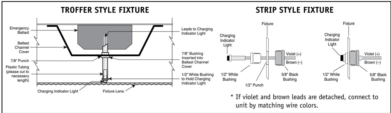
NOTE: After installing the charging indicator light and test switch, mark each with the appropriate label.
