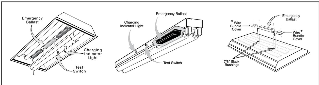
\*For installation on top of the fixture, wire bundle covers may be required by state or local codes. These covers are available from the manufacturer as an accessory kit and must be ordered separately. Call your local distributor or the factory for complete information.
