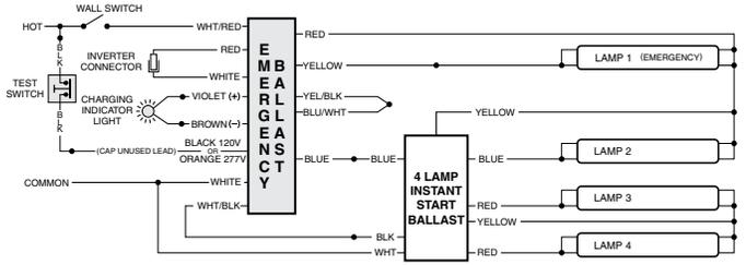
FIG H FOUR (4) LAMP RAPID START BALLAST
