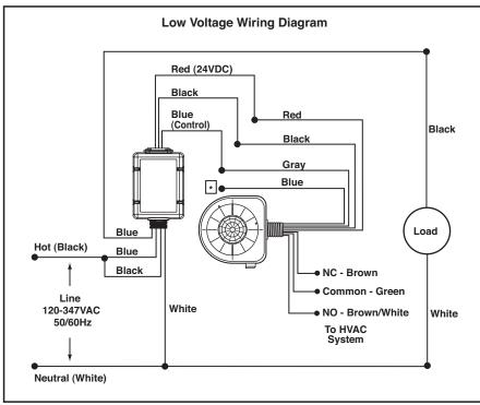
\* Note: The blue wire is only to be used when you DO NOT want to use the daylight (photocell) feature. Connect the blue wire instead of the gray wire to the blue wire on the power pack.
