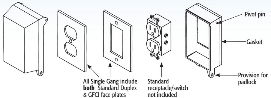
Arlington's DRI-BOX<sup>®</sup> Adapter comes with both standard duplex and GFCI plates for added convenience, but works with any standard plastic or metal wall plate. Our DRI-BOX<sup>®</sup> meets OSHA lockout/tagout requirements using a standard padlock.
