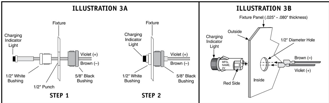
**NOTE:** After installing the charging indicator light and test switch, mark each with the appropriate label. If a detached charging indicator light is used, connect by matching wire colors and install as shown above.
