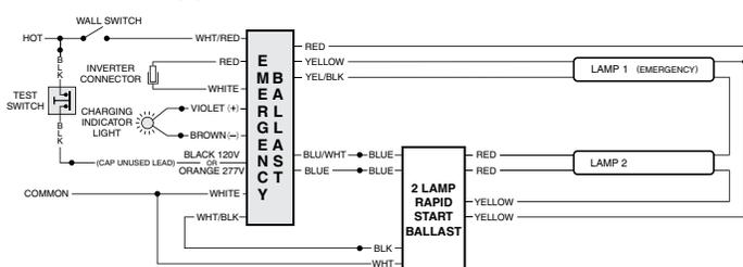
**FIG L TWO (2) LAMP PROGRAM RAPID START OSRAM BALLAST**
