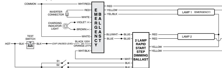
THE WHITE/BLACK LEAD MUST CONNECT TO THE WHITE LEAD OF THE STEP-DIMMING BALLAST ASSOCIATED WITH THE EMERGENCY BALLAST ONLY. CONNECTIONS TO OTHER BALLASTS OR FIXTURES COULD RESULT IN ABNORMAL OPERATION AND CAUSE PRODUCT DAMAGE.
