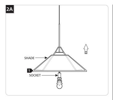
1 Lift the shade up to expose the socket.
