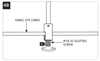
Place the power feed connectors onto each Kable Lite cable. Replace and tighten the #8-32 slotted set screw.
