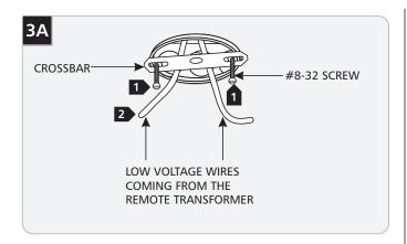
**NOTE:** Low voltage wires must be present in electrical box before proceeding with these steps. Refer to the instructions provided with the remote transformer.
