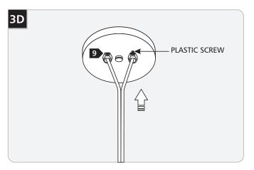
Push the excess power feed wires into the canopy and tighten the plastic screw.
