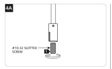
1 For each power feed connector remove the #8-32 slotted screw with a flat head screwdriver.
