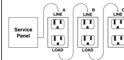
Placing the GFCI in position A will also provide protection to "load side" receptacles B and C. On the other hand, placing the GFCI in position C will not provide protection to receptacles A or B. Remember that receptacles A, B, and C can be in different rooms.
