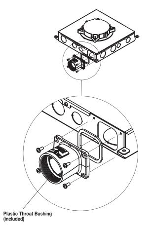
CAUTION: Ensure plastic throat bushing is inserted in place in front of conduit thread
