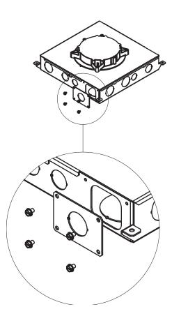
**Step 2.** Position gasket between 2-inch conduit hub fitting and floor box and mount conduit hub fitting with (4) #10-32 x 7/16 in. screws provided. Tighten screws to 2 ft-lbs. (3 N-m).
