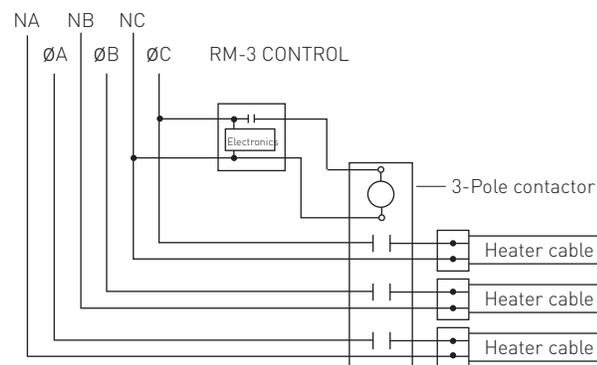
**Figure 18 Typical wiring diagram using a RM-3 controller—multiple circuits**
