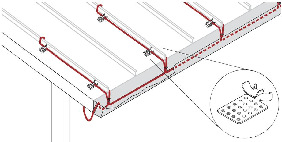
**Figure 13 H913/H914 clip on standing seam roof**
