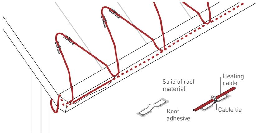
**Figure 14 Belt loop approach on a sloped roof**
