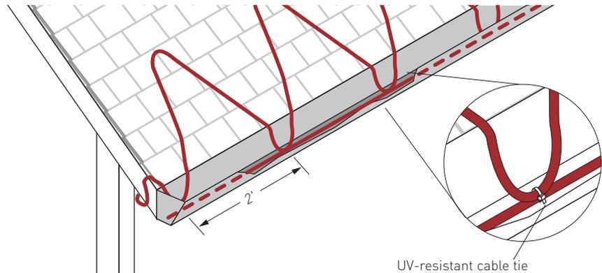
**Figure 3** Layout in a serpentine pattern
