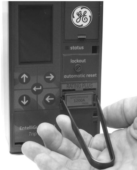
Figure 2. Rating plug removal
