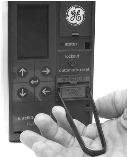
Figure 2. Rating plug removal
