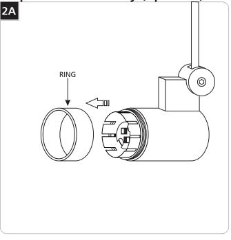
If installing a head accessory, pull the ring off of the fixture.
