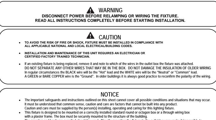
The crossbar and hardware supplied should be used. Directly mounting the fixture to the outlet box may make it impossible to correctly align the fixture
