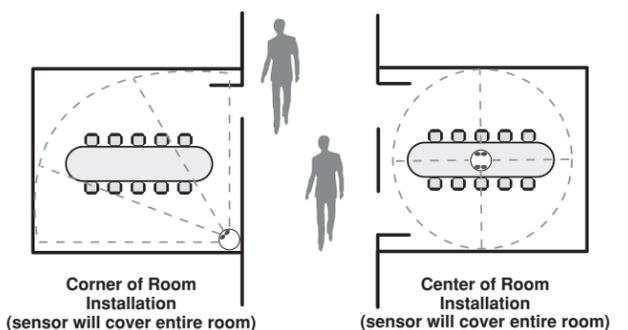
**NOTE:** When mounting device, do not point sensor openings towards the opening of a door or strong air currents.
