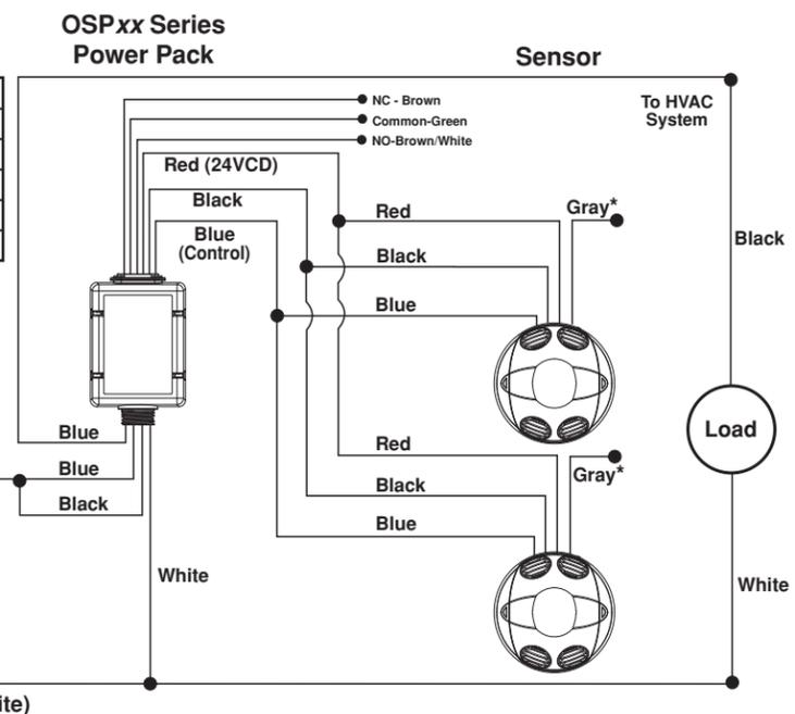
**\*NOTE:** When using the Photocell function, connect the Gray wire of the sensor to the Blue wire of the power pack. **DO NOT** use the Blue wire of sensor.
