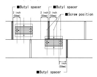
• When there are gaps in the position to install, cut butyl tape in the shape of the gap and place it.
