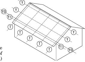
(iii) Line Y: Center of brackets of the second and after rows. The distance between Y1-Y and Y-Y shall be the width of panel (see figure of previous page) plus 1-3/16 inch (30 mm, equivalent to the width of a Panel Spacer).
