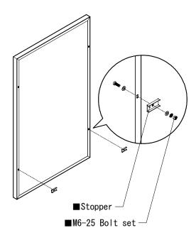
③ The stopper is to be installed on the panels of the lowest row only.
