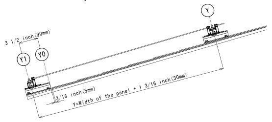
(iv) Line T: Line delineate the edge of a panel or center line of the gap between consecutive panels. The distance between T Lines shall be the length of a panel (see figure of previous page) plus the gap width. The gap width of 1/8 inch (3 mm) is recommended, but any other width you prefer can be used.
