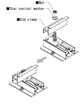
② Installation steps for the stopper (The panel stopper allows the installer to quickly align the array up when the bottom brackets are perfectly lined up.)
