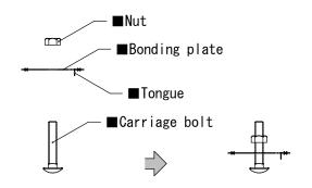
② For the middle column clamps: Preassemble the Carriage bolt with the Bonding plate, Spacer, Star conical washer and Hex Nut per illustration.
