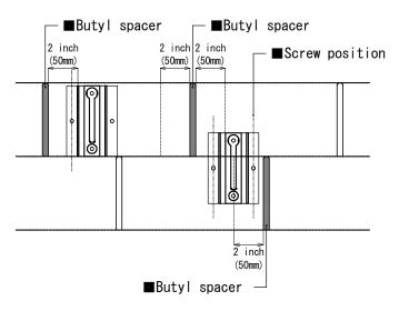
• When there are gaps in the position to install, cut butyl tape to the shape and place it.
