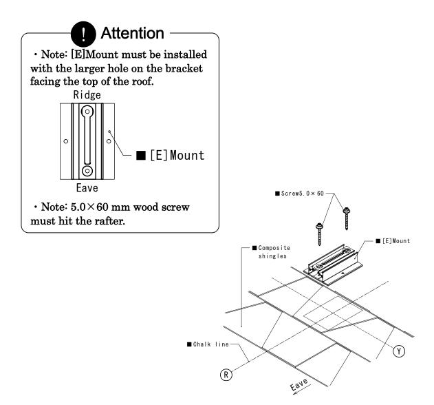
Apply roof sealant around the brackets, the top and each side edge of the brackets.
