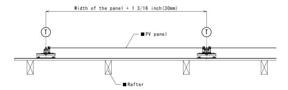
② Position the brackets. Make a chalk line according to the PV module installation instruction.
