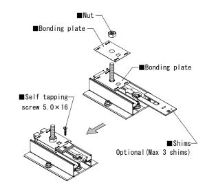
The Set the carriage bolt and nut to torque 110 in-lbs (12 Nm).
