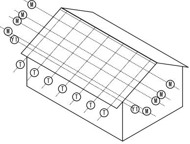
(i) Line M: Bracket center line. Refer to the PV panel manufacturer's instruction for adequate installation area.
