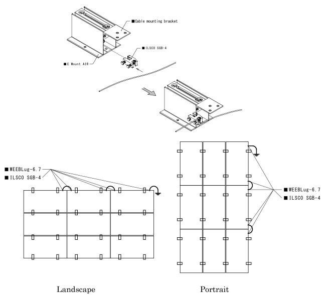
In order to properly ground the PV modules and the brackets to the equipment ground, a grounding lug or lay-in lug must be attached to the PV module at the end of each row.
