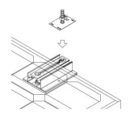
③ Place the End clamp and tighten it to 110 in-lbs (12 Nm).
