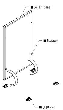
$\ensuremath{\$}$  Place the PV panel on the bracket.
