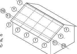
(iii) Line Y: Center of brackets of the second and after rows. The distance between Y1-Y and Y-Y shall be the width of panel (see figure of previous page) plus 1-3/16 inch (30 mm, equivalent to the width of a Panel Spacer).
