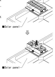
Slide the panel spacer until it is flush to the panel frame.
