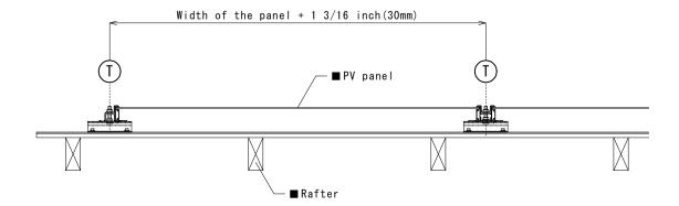
② Position the brackets. Make a chalk line according to the PV module installation instruction.
