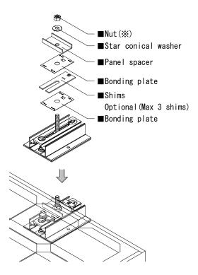
When shims are used for leveling, set the self tapping screw  $5.0 \times 16$  through the shims.
