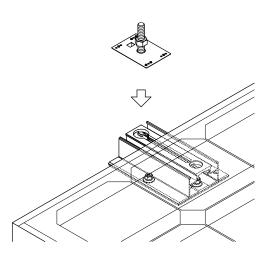
③ Place the End clamp and tighten it to 110 in-lbs (12 Nm).
