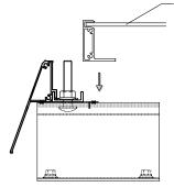
Set the Middle clamp in order to support the positioning of the panel being placed down.
