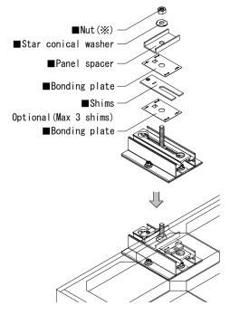
③ When shims are used for leveling, set the self tapping screw 5.0 × 16 through the shims.
