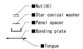
② For the middle row brackets and clamps & the bottom end brackets and clamps with the Skirt option installation: Carriage bolt, Bonding plate, Spacer, Star conical washer and Nut.
