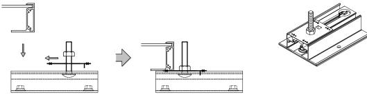
If shims (3 max.) are to be used to level the brackets, another bonding plate shall be added right on top of the shims.
