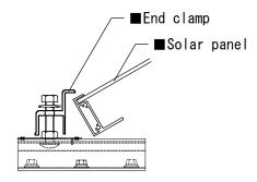
9 Make any adjustment and tighten the nut to 110 in-lbs (12 Nm).
