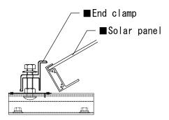
8 Make any adjustment then tighten the nut to 110 in-lbs (12 Nm).
