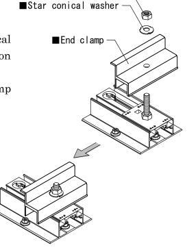
⑥ Installation steps for the stopper (The panel stopper allows the installer to quickly align the array up when the bottom brackets are perfectly lined up.) Tighten the M8 bolt.
