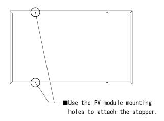
The stopper is to be installed on the panels of the lowest row only.
