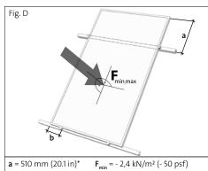
$F_{max} = + 5.4 \text{ kN/m}^2 (+ 113 \text{ psf})$
