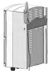
Figure 4: Routing the antenna cable
