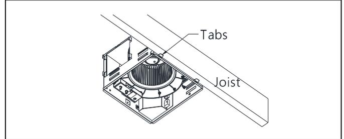
2. The housing mounts with 4 long wood screw (ø4x25). Screw housing to joist through lowest holes in each mounting flange, then through the other holes.
