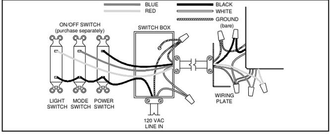
4. Using wire nuts (not provided), connect house power cable to ventilating fan.
