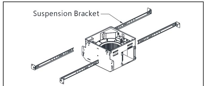
4. Extend suspension brackets to the width of the joists. Make sure the fan body is level and perpendicular with the joist.
