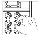
Next, plug in and turn ON the lamp or radio at the receptacle's other outlet to make sure the power is OFF at both outlets. If the power is not OFF, stop work and call an electrician to complete the installation.
