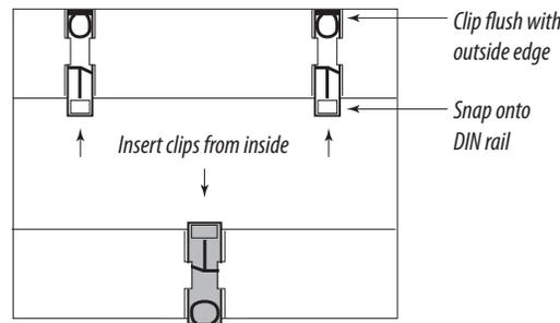
3. To reduce horizontal shifting across the DIN rail, use two end stop clips.
