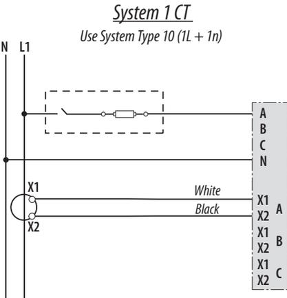
*Diagram 2: 1-Phase Line-to-Line 2-Wire*
