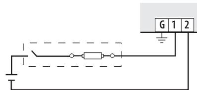
DC Control Power from 125 VDC to 300 VDC (UL and CE max.)
