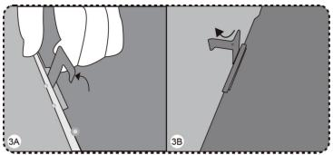
**4.)** After securing the product on the T-bar with hang buckle (as shown in diagram above), secure panel to the ceiling with aircraft cable or wires capable of supporting 100lbs minimum.
