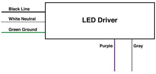
\*\* 0-10v IEC dimming Control wires
