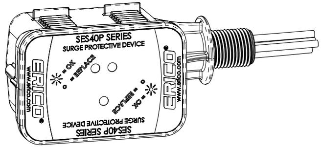
**⚠ CAUTION** CAUTION: Ungrounded power systems are inherently unstable and can produce excessively high line-to-ground voltages during certain fault conditions. During these fault conditions any electrical equipment, including an SPD, may be subjected to voltages which exceed their designed ratings. This information is being provided to the user so that an informed decision can be made before installing any electrical equipment on an ungrounded power system.
