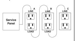
Placing the GFCI in position A will also provide protection to "load side" receptacles B and C. On the other hand, placing the GFCI in position C will not provide protection to receptacles A or B. Remember that receptacles A, B, and C can be in different rooms.
