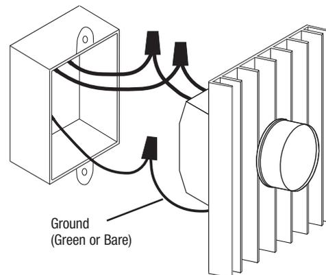
4. Push wires into wallbox, allowing room for dimmer backcover to be inserted.
