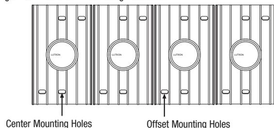
**5.** Snap multiple single wallplates onto controls and adjust up or down for a snug fit. See Figure F.
