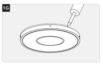
For wet location installation, caulk around the mounting base with waterproof construction sealant.
