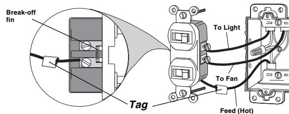
**Step 4** Disconnect switch wires.
