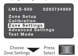
When Zone Settings is selected, one of two screens is displayed depending on the Operation Mode of the Zone (Switched) or (Dimming, Bi-Level or Tri-Level):
