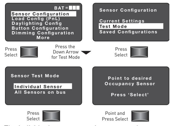
The individual sensor goes into test mode.
