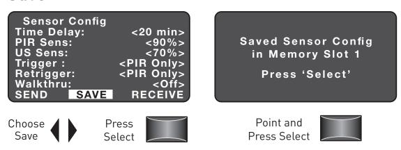
This saves the settings in the LMCT-100 "Saved Configurations" menu function for future use. Each time you save a configuration the "Memory Slot" number increases. You can save up to 9 configurations. Saved configurations are listed in the LMCT-100's "Saved Configurations" function in the Sensor Configuration menu (for more details, see page 12).
