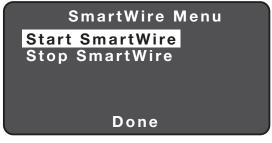
Press Select With Start Smartwire selected, point the LMCT at the switch or sensor to be programmed and press **Select** to enter the Smartwire mode. Select **Stop Smartwire** and point at the device to exit the Smartwire mode.
