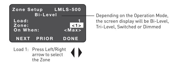
For Bi-level and Tri-level only, press the Down arrow for On When to appear.
