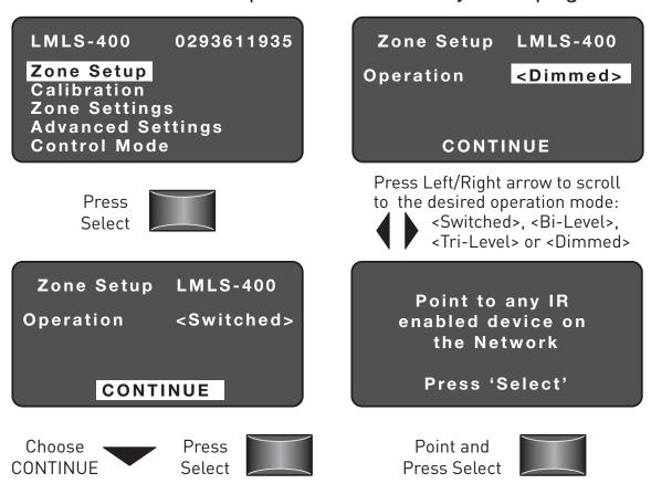
After choosing Zone Setup and pressing Select, the current operation mode is displayed. This can be changed to Switched, Bi-Level, Tri-Level, or Dimmed.
