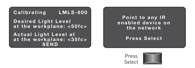
To set the Dimming and On and Off Setpoints automatically to best match a designed light level for the workplane, enter the desired level, along with the present measured level (from a light meter), and then press SEND.
