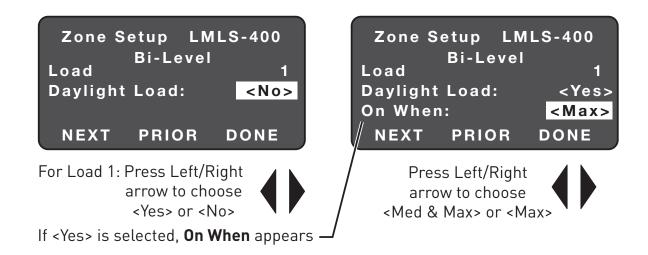
To do load binding the load needs to be assigned as a Daylight Load by selecting <Yes>.
