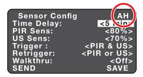
**Explanation:** There are two sets of parameters in every device, one for normal hours, which is the default configuration, and one for After Hours. "AH" is a flag that appears on a screen if the device that the LMCT-100 is communicating with is in After Hours mode.
