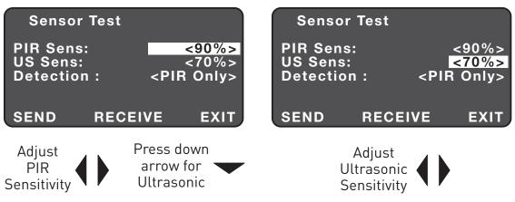
You can adjust sensitivity values while inside the Test Mode. Values are 0 to 100%, in 10% increments.
