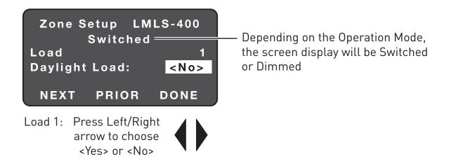
To do load binding the load needs to be assigned as a Daylight Load by selecting <Yes>.
