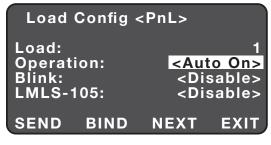
Operation Mode <Manual On> or <Auto On> The operation mode determines if the load can be turned on automatically by a sensor, or only manually by a switch. Push
