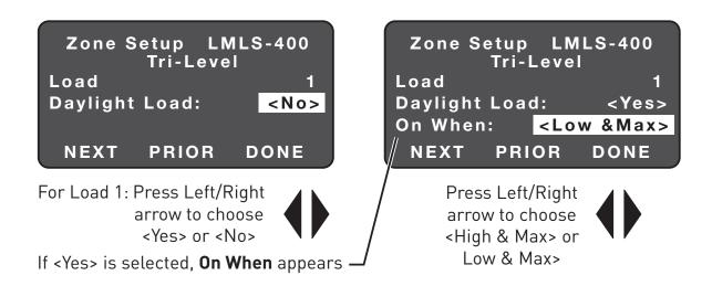
To do load binding the load needs to be assigned as a Daylight Load by selecting <Yes>
