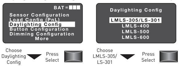
Refer to the LMLS-305 installation instructions for details about daylighting setup and operation.
