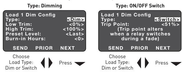
Important: All loads connected to dimming capable room controllers default to Load Type <Dim>. Be sure to select the appropriate load type because these room controllers can control either type of load. Default settings are based on the load type selected.
