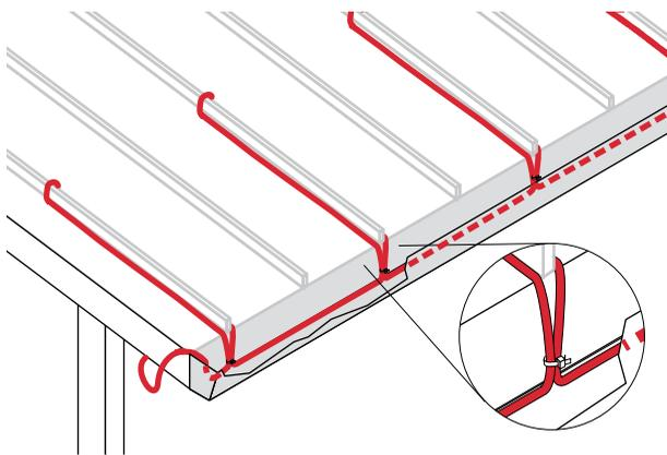
Figure 6: Layout on a standing seam roof
