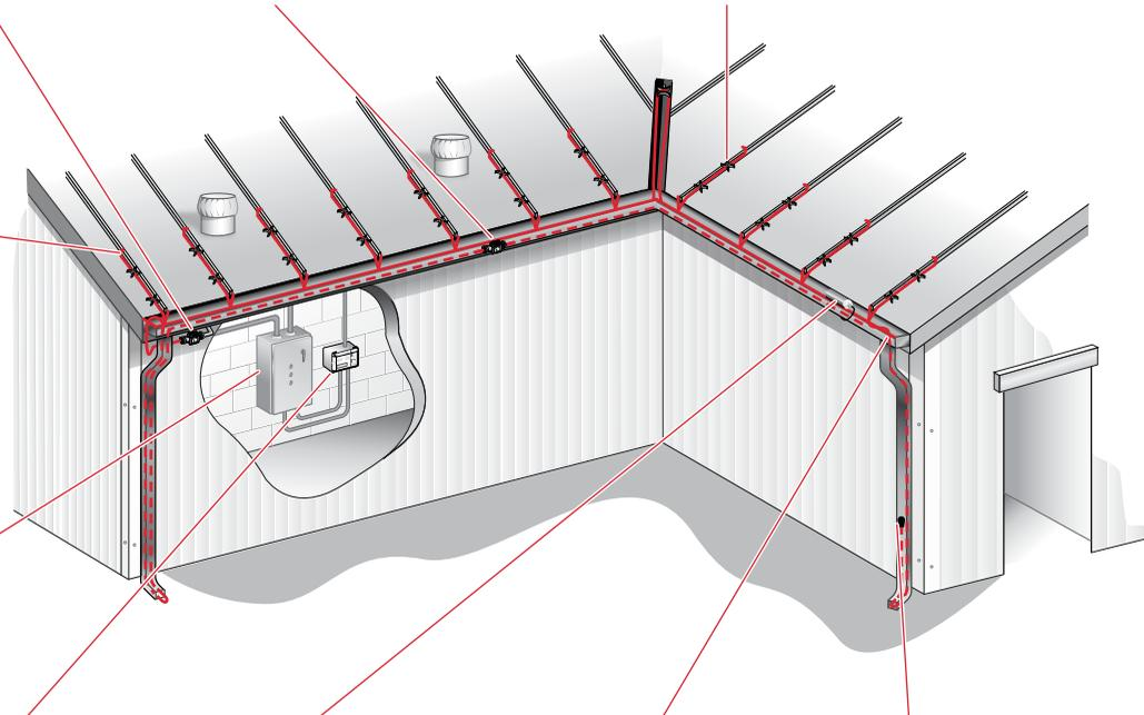
Figure 1: IceStop Roof and Gutter De-Icing System
