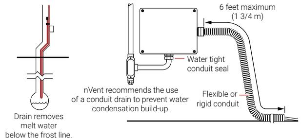
**Figure 14: Installation of IceStop cable in trench drains**
