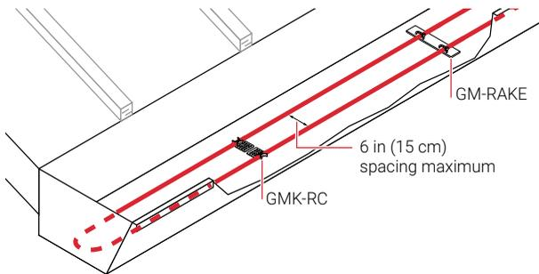
**Figure 13: Layout in wide gutters—6 to 12 in wide**
