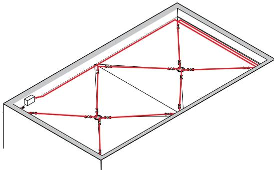
Figure 21: Belt loop approach on a flat roof
