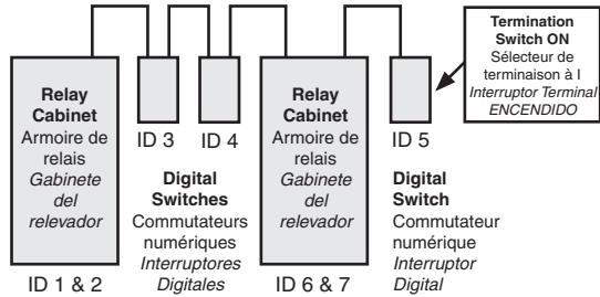
Digital switches are powered from the relay cabinet. Termination switch is set to ON in digital switch ID 5 and on Command Module, all other termination switches are in the OFF position.
