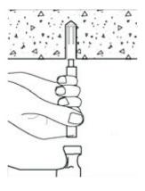
blows until the shoulder of the tool is seated against the anchor. Anchor will not hold allowable loads required if shoulder of *Powers* setting tool does not seat against anchor.
