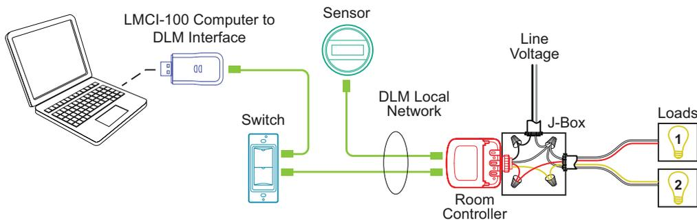
**CAUTION: TO CONNECT A COMPUTER TO THE DLM LOCAL NETWORK USE THE LMCI-100. NEVER CONNECT THE DLM LOCAL NETWORK TO AN ETHERNET PORT – IT MAY DAMAGE COMPUTERS AND OTHER CONNECTED EQUIPMENT.**
