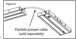
inserting fully. The maximum number of units that can be interconnected is based on total wattage. Do not exceed the maximum of 150 watts connected to a single dimmer; or with one power cord; or linked together, either with jumpers or directly.
