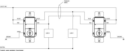
LIGHTS WILL TURN OFF, WHEN UNIT THAT WAS TURNED ON LAST AND/OR DETECTED MOTION LAST TIMES-OUT
