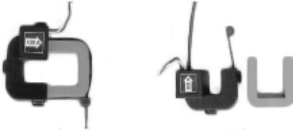
Fig. 3. Split-Core Current Sensor Assembly
