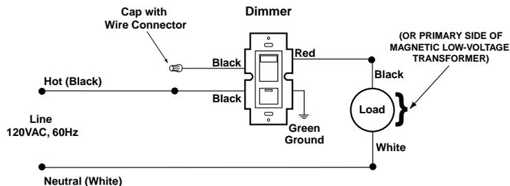
Wiring Diagram 2 - Two Location Control Application
