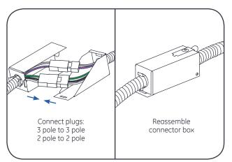
**6** Connect the two quick connectors and reassemble the connector box.
