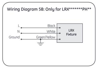
**NOTE:** Phase cut dimmer has to be fixed on hot line (L). Dimming compatibility refer to GE website.
