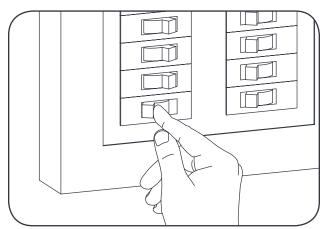
**2** Ensure that the power to the unit is turned off. Use proper lockout and tagout procedures.
