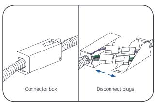
4 Disassemble the connector box and unplug the two quick connectors inside.
