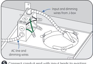
5 Connect conduit end with input leads to existing junction box and make proper connections. Connect the black, white, and green/yellow wires of the input leads to the black, white and green wires using twist-on wire connectors and close junction box.
