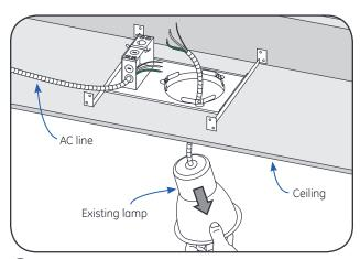
3 Remove existing lamps, fixture and ballast. Leave wiring in junction box. Verify that the AC supply line is provided with a ground wire connected to the luminaire.
