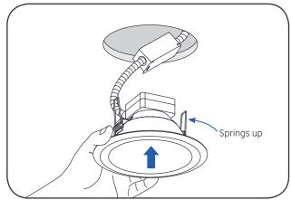
**7** Load springs into upright position by twisting the springs upward and carefully insert the fixture to the hole of the frame. Verify reflector trim is flush with ceiling.
