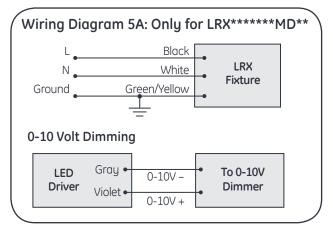
**Optional dimmer:** When connecting with dimming controller, wires must be run through another separate knockout hole. Connect the violet (dimming +) and gray (dimming -) wires to the violet and gray wires of the fixture.
