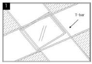
Place one end of the product on the T-bar. To secure the luminaire (fixture) position in ceiling, squeeze tabs into T-bars to lock luminaire (fixture).
