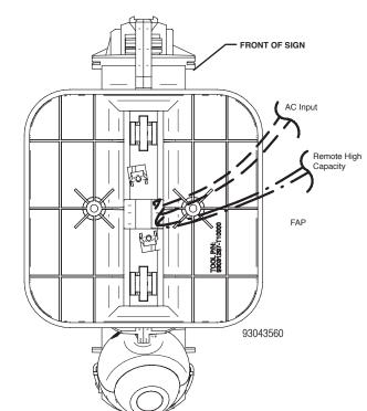
The EVC sign is designed to be wall, ceiling or end mounted. Provide standard and Spectron® equipped signs with single un-switched supply from a 120 or 277VAC branch circuit used for normal lighting in the area to be protected.
