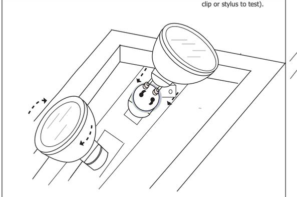
Slide fixture head onto the heads of the two socket head bolts until flush with wall or ceiling surface.
