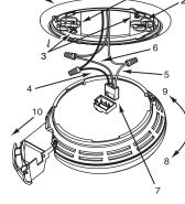
The Parts of This Unit Mounting Bracket Mounting Slots Locking Pins (break out of bracket) Hot (Black) AC Wire Neutral (White) AC Wire 6 Interconnect (Orange) Wire Quick-Connect Power Connector 3 Turn this way to remove from bracket 9 Turn this way to attach to bracket
