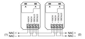
Polarity is shown in the active state.
