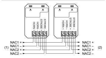
Polarity is shown in the active state.
