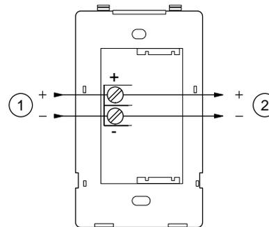
1. From compatible fire alarm control panel
