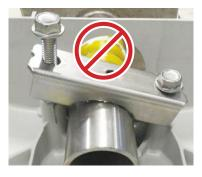
WARNING: Avoid tightening bolts unevenly, as it may cause cross-threading.
