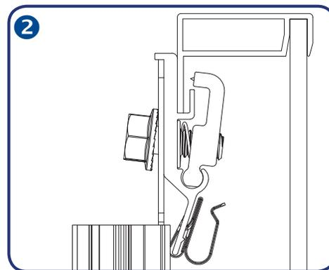
3. Tighten the mounting bolt on the MLPE Frame Attachment Kit to 10 lb-ft (120 lb-in).
